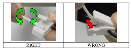
Figure 23. Brush softly the sensor with the cotton.
