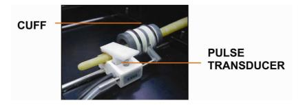
Figure 18. Cuff and Transducer placing in the tail.
