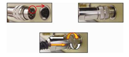
Figure 17. Connecting and disconnecting transducer.
