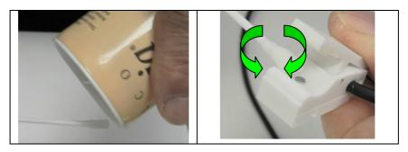
Figure 24. Rotating brush with cotton covered with talcum powder.
