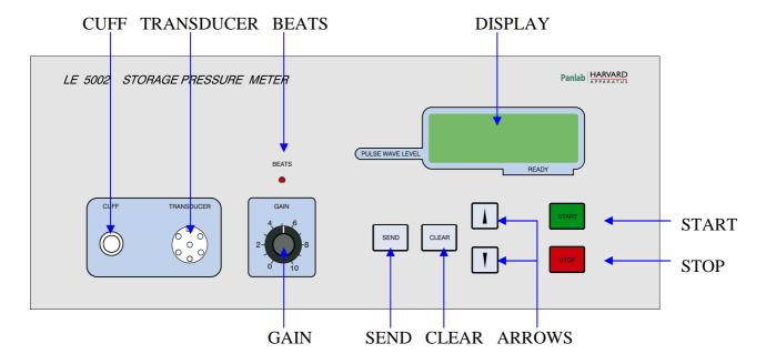
Figure 7. Control Unit Front Panel.
