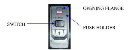
Figure 1. Power inlet, main switch and fuse holder.
