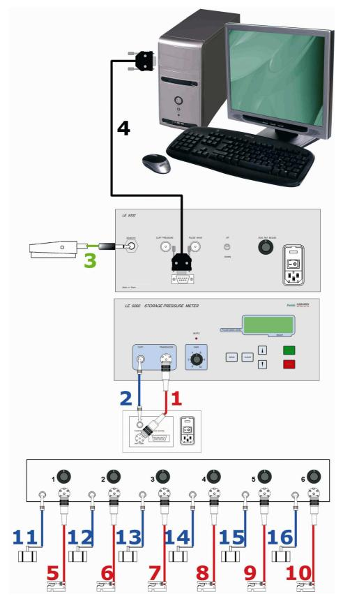
Figure 11. Connection between LE 5002 and LE 5650.
