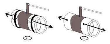
Figure 26. Removing O rings and membrane.
